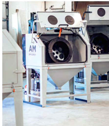
At left: Ulf Qviberg (right) and his team At right: Along with the usual powder-removal features, AM Efficiency integrates surface smoothing into its systems
