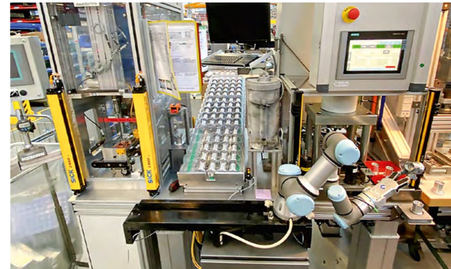
Above: A lot of 3D Printing in a small space: For this production station, an entire ball bearing feeding machine, the 40 cm frame of an inspection station and a depositing platform were printed in PA12 along with a gripper made of titanium.
