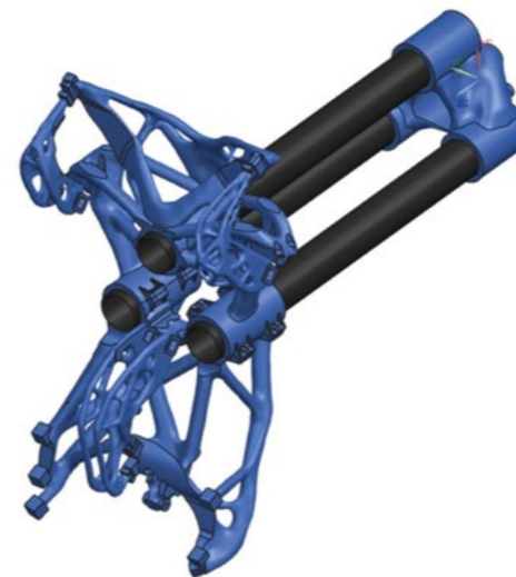
Above: Thanks to their reduced weight, 3D printed brackets can lower an aircraft's carbon emissions by more than 43 tons compared to conventionally produced (and designed) parts Below: Designs with optimized topology can also make significant weight reductions possible in 3D printed robotic grippers. This ultimately makes robots more efficient, as well
