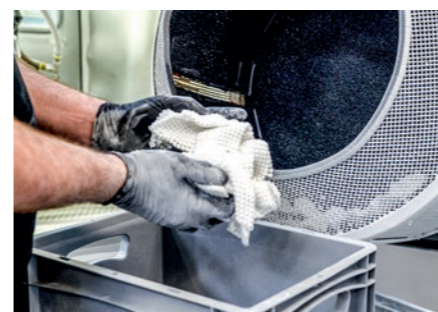
Photo above: The parts when being unloaded from the Powershot C (Cleaning).
